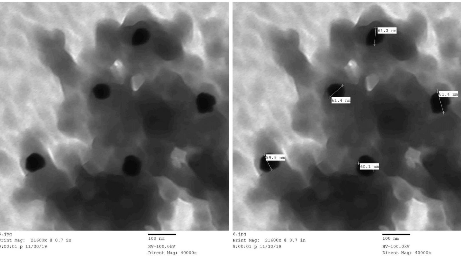
**Fig.(2):** Electron micrograph of AuNPs suspension on Transmission Electron Microscopy (TEM) showing majority of almost spheroidal to rod shaped gold nanoparticles with diameters ranging between 59.9:81.4 nm.
