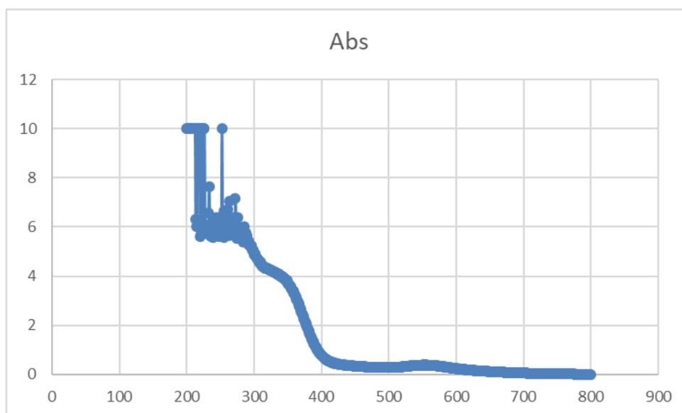
**Fig.(1): AuNPs were examined by UV/VIS spectrophotometer Particles absorbance was maintained at range between 200:800 nm.**
